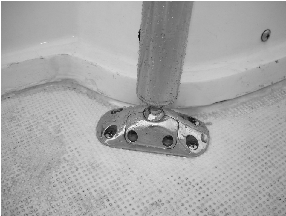
Swivel Feet: Swivel feet can pitch match the crown in your deck. They also turn to any angle, as shown above, to best fit close to your console. And they allow removal of the Ttop from the boat for storage without disturbing the actual deck mounting fasteners. Note the cap is to the outside.
